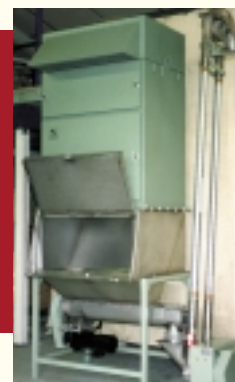
Vertical conveyor feed from sack tipping station with screw feeder outlet and integral dust extraction system.
