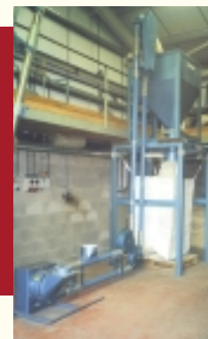
Horizontal/vertical multi-path conveyor.
