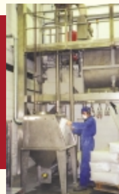
Manual sack tipping into mixer using vertical conveyor and integral feed screw.
