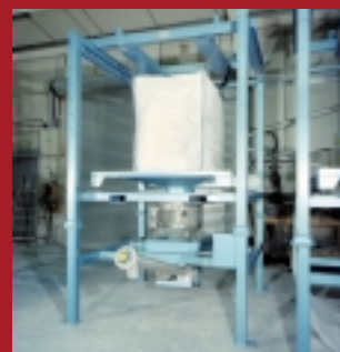
'Bagstander' FIBC Discharge System
